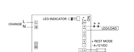
Wiring diagram - Non-maintained (emergency only)
